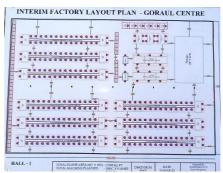
It can be seen that all the functional units and subunits are placed in distinct locations one after the other so that the operation of a unit doesn't interfere with that of another unit.
